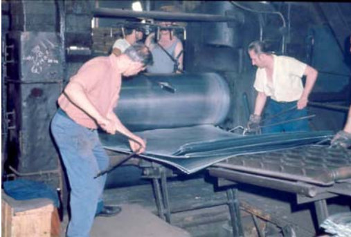
Fig. 6: Production of sheets of zinc using the pack rolling process
