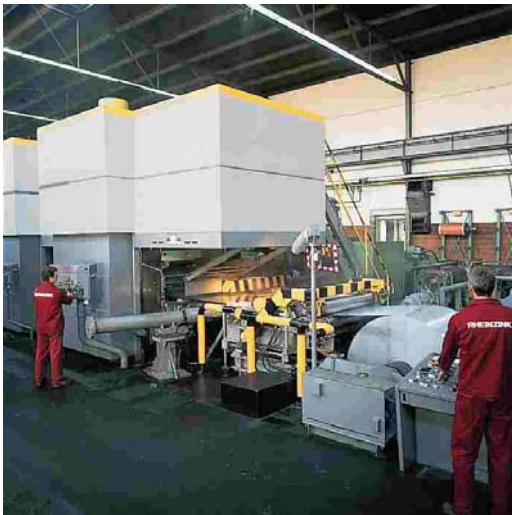
Fig. 14: At the end of the rolling train the finished strip is wound into large coils and stored temporarily for cooling.
